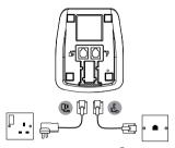
2. Plug the power adaptor into the socket marked 🗓 on the rear of the base and plug the other end into the mains power wall socket. Switch on the mains power.
